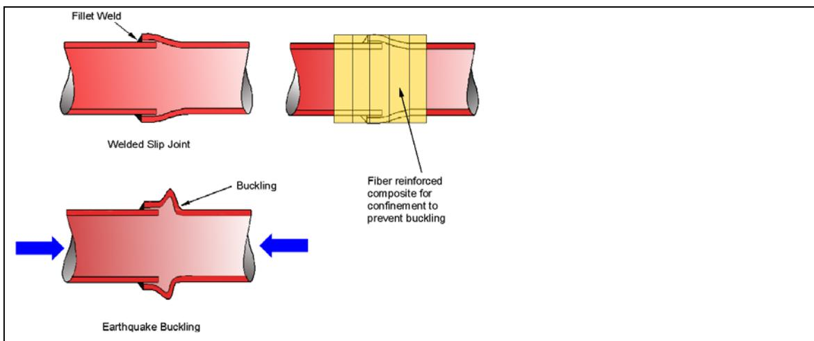
confine and strengthen welded slip joints against seismic compressive forces. Welded slip joints retrofitted with FRP technology restore pipelines to their full strength, as if they were straight sections without joints. This type of reinforcing can be used not only to retrofit existing welded slip joints, but also to strengthen new joints during fabrication in the field. The FRPs are now commercially available from several companies.
