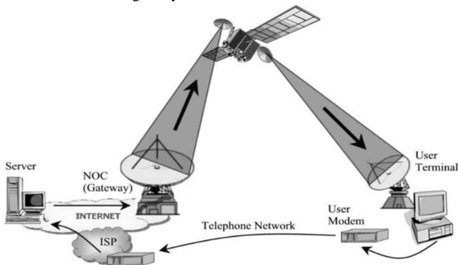
*The original DirecPC system was a novel hybrid of satellite and telephone network links.*
