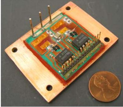
drives. Embedded power technology has been adopted to eliminate all wire bonds in favor of a planar interconnection scheme that minimizes dangerous voltage transients caused by unwanted parasitic inductances. In addition, the flat upper surface is valuable for mounting gate drives, sensors, and cooling components to extract extra heat from the top side of the module. Such advances contribute to reducing the module size while increasing its long-term robustness.
