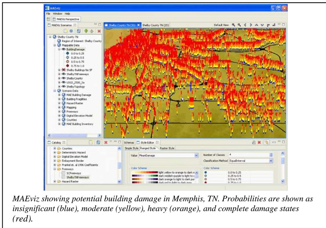
*MAEviz showing potential building damage in Memphis, TN. Probabilities are shown as insignificant (blue), moderate (yellow), heavy (orange), and complete damage states (red).*
