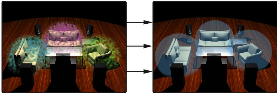
*Loudspeakers in a typical stereo or surround-sound system interact with surfaces to produce audible distortions at each listening position. MultEQ reduces the effects of the distortions, providing an enhanced, more uniform listening experience for everyone.*
