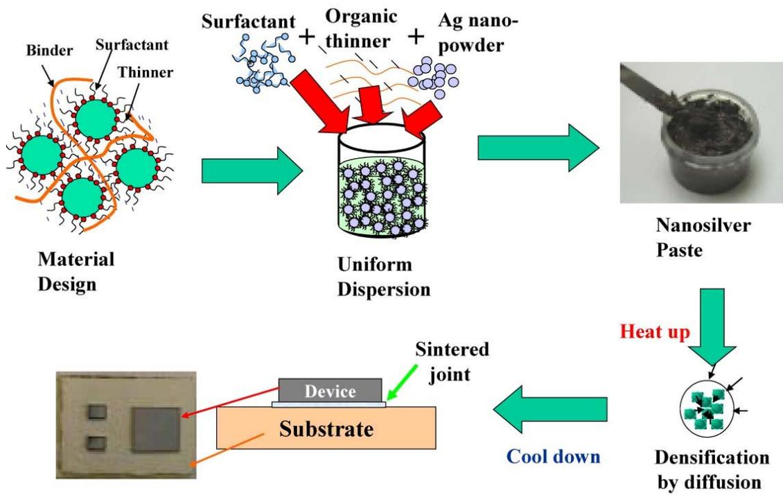
*Process for production of NBE Technologies' nanosilver paste product, being commercialized as nanoTach.*
