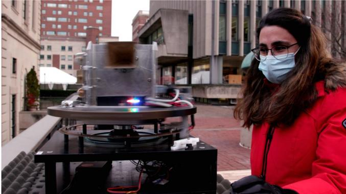
*Columbia Engineering students take millimeter wave channel measurements for the COSMOS advanced wireless research testbed in West Harlem. COSMOS is a cloud-enhanced open software defined mobile wireless testbed for city-scale deployment. (Credit: Columbia Engineering)*
