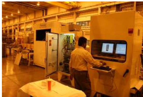
An operator inspects the images of an engine block in which pores were detected and makes the intelligent decision whether the engine block is indeed defective.
