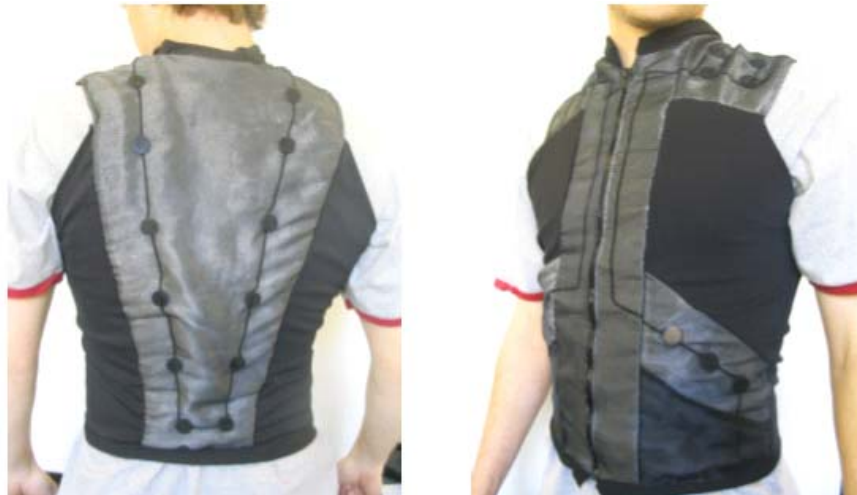
VibeAttire's motors are removable so that the garment can be washed.
