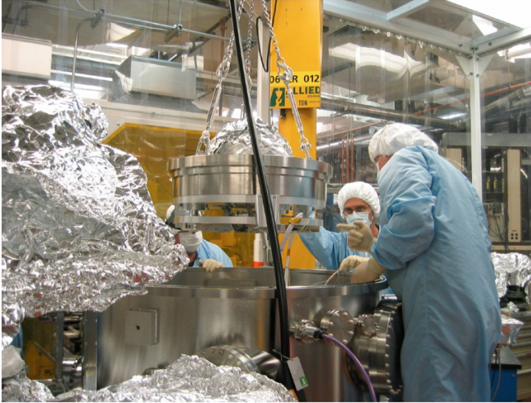
Sematech-supported Micro-Exposure-Tool (MET) optics being installed at UC-Berkeley (an ERC EUV partner) for EUV photoresist and mask defect printability testing.
