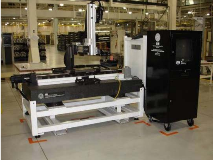
The ERC/RMS Reconfigurable Inspection Machine is inspecting engine blocks on a Chrysler production line in Dundee, Michigan
