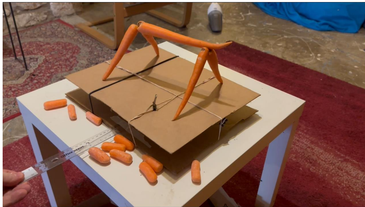
FIGURE 5-3 Still from the Example 3: Earthquake Shake Table video.
