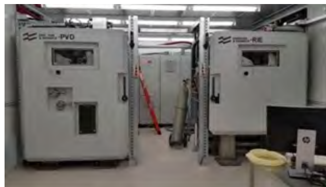
Figure 6-6: NASCENT's roll-to-roll (R2R) nanofabrication line can etch a variety of inorganic materials and metals. (Photo credit: The University of Texas at Austin)
